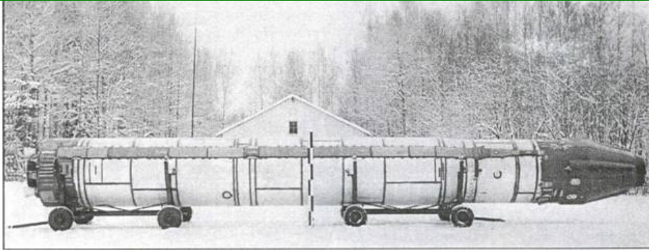
ICBM RS-16A assembled without warhead (outside the launch container)
